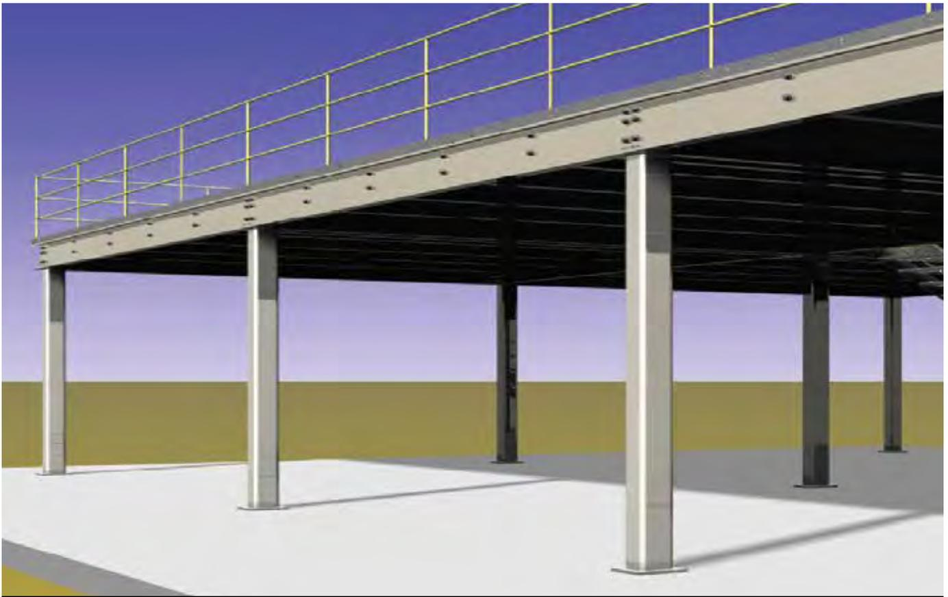
**Figure 4.** Example of a cold-formed steel–special bolted moment frame.
