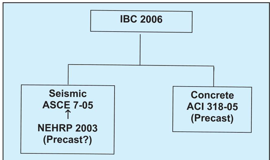
Fig. 6. Seismic design provisions for precast concrete structures in the 2006 IBC.
