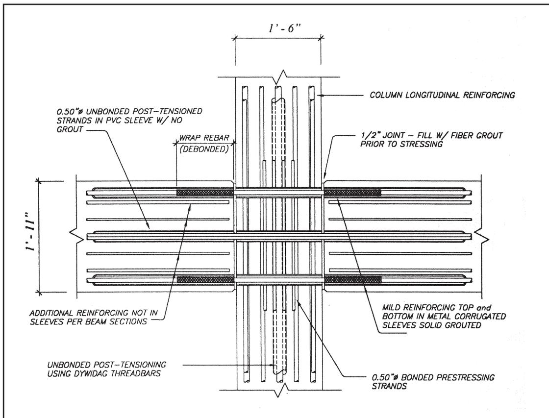
Fig. 1. Idealization of interior column hybrid connection used in the PRESS Test Building (transverse joint reinforcement not shown for clarity only).
