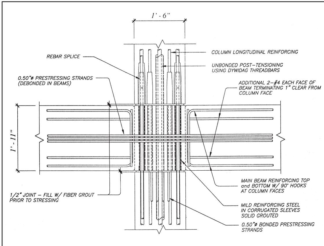
Fig. 2. Idealization of interior column pretensioned connection used in the PRESS Test Building (transverse joint reinforcement not shown for clarity only).
