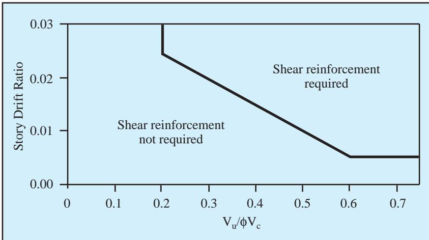
Fig. 3. Punching shear reinforcement requirements at flat plate-column joints.
