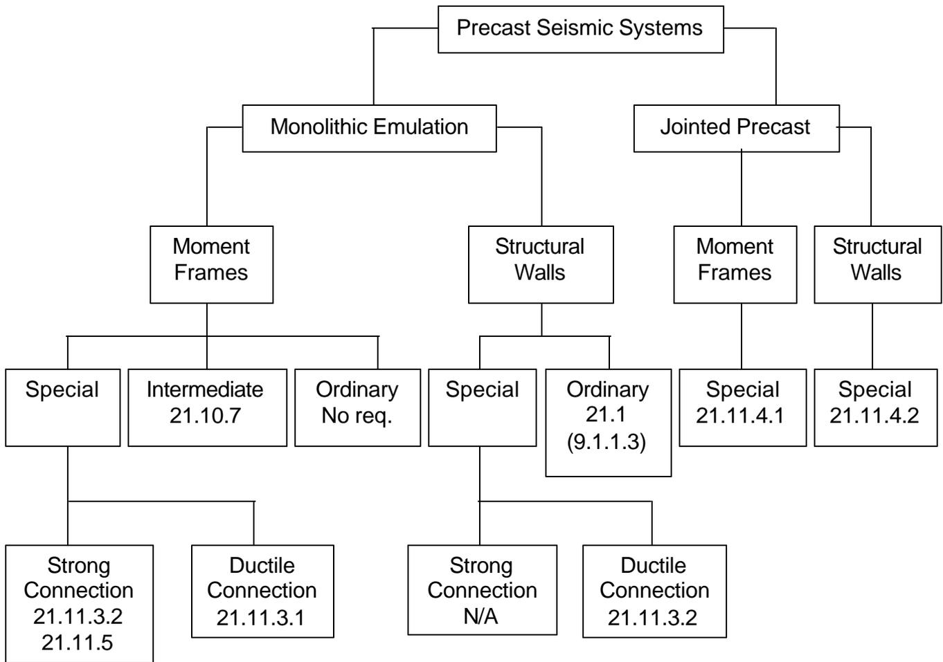
**Fig. 1: Seismic design requirements for precast structures in 2000 NEHRP Provisions**
