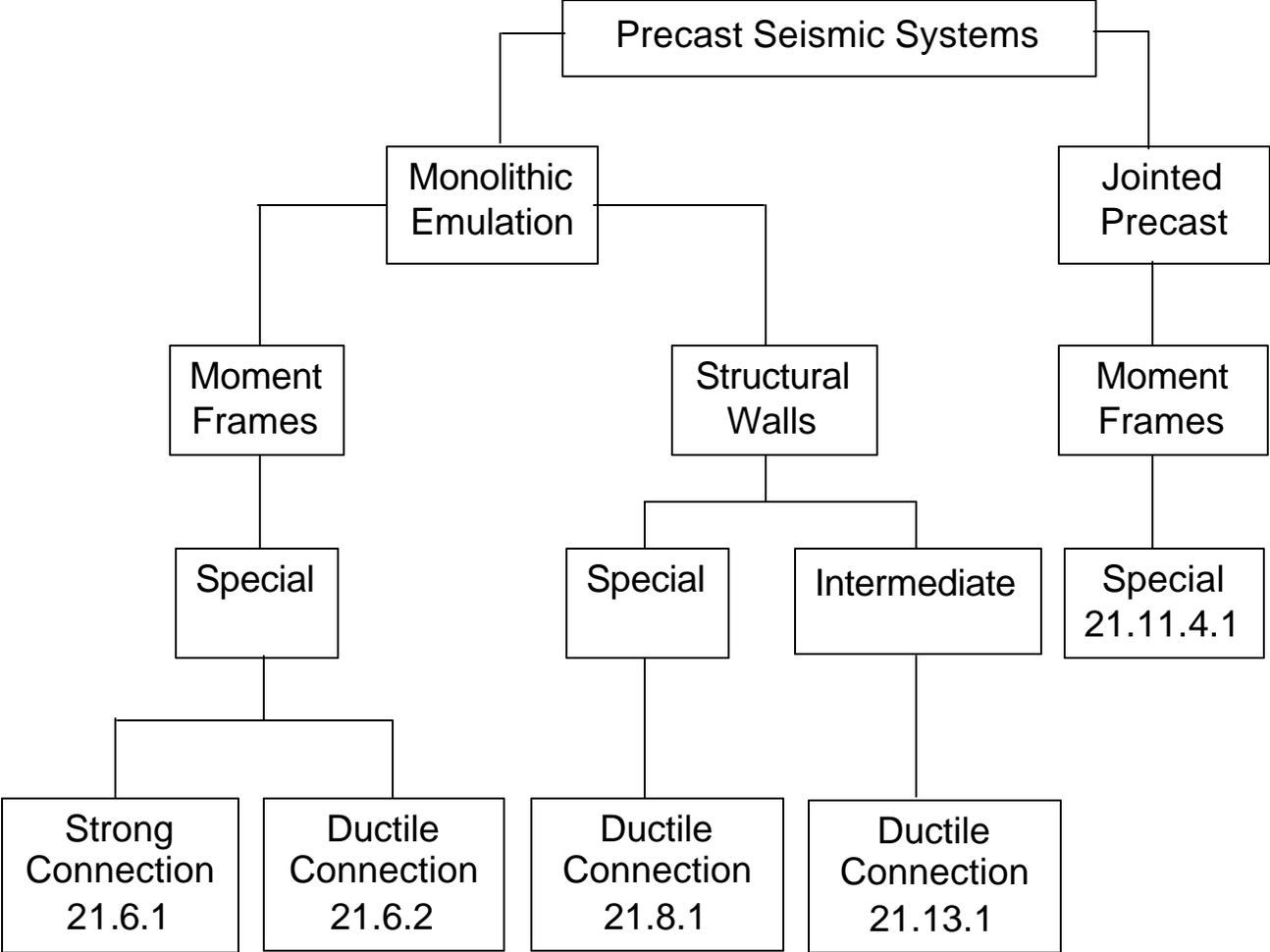
**Fig. 2: Seismic design requirements for precast structures in ACI 318-02 (expected)**
