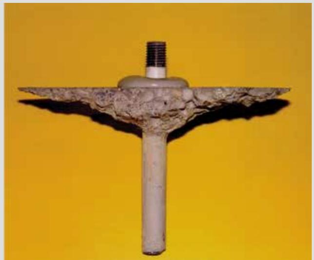
**Figure 5.** Adhesive anchor and bond failure of adhesive anchor. Photo courtesy of Rolf Elgehausen, University of Stuttgart.
