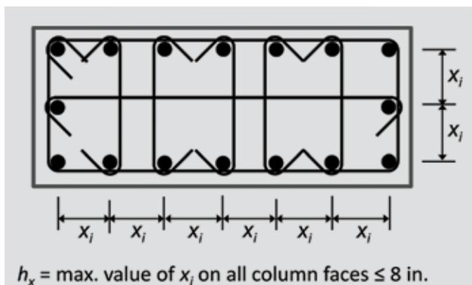
**Figure 5.** Confinement of high-strength or highly axially loaded rectangular column of special moment frame. Note:  $d_b$  = nominal diameter of bar, wire, or prestressing strand;  $h_x$  = maximum value of  $x_i$  on all column faces greater than 8 in.;  $x_i$  = dimension from centerline to centerline of laterally supported longitudinal bars. 1 in. = 25.4 mm.
