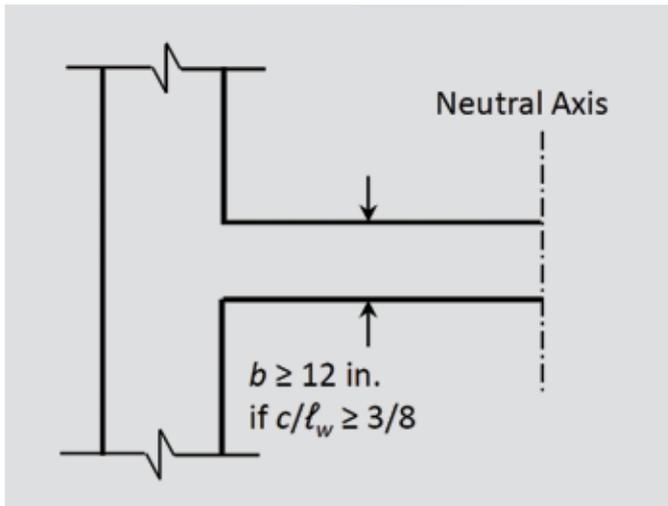
**Figure 10.** Minimum thickness of compression zone of special shear wall that is not tension controlled. Note:  $b$  = width of compression face of member;  $c$  = distance from extreme compression fiber to neutral axis;  $l_w$  = length of entire wall or length of wall segment or wall pier considered in direction of shear force. 1 in. = 25.4 mm.
