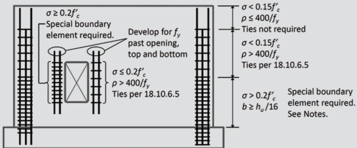
Notes: Requirement for special boundary element is triggered if maximum extreme fiber compressive stress  $\sigma \geq 0.2f'_c$ . Once triggered, the special boundary element extends until  $\sigma < 0.15f'_c$ . Since  $h_w / \ell_w \leq 2.0$ , 18.10.6.4(c) does not apply.
