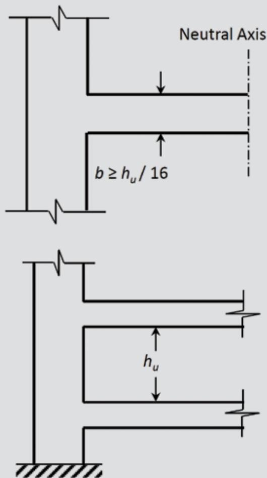
**Figure 12.** Minimum thickness of compression zone of special shear wall. Note:  $b$  = width of compression face of member;  $h_u$  = laterally unsupported height at extreme compression fiber of wall or wall pier, equivalent to  $\ell_u$  for compression members;  $\ell_u$  = unsupported length of column or wall.
