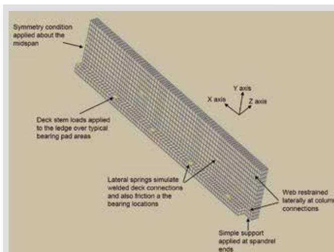
**Figure 2.** Finite element model of a precast concrete spandrel beam. Image from Lucier et al., “Development of a Rational Design Methodology for Precast Concrete Slender Spandrel Beams: Part 2, Analysis and Design Guidelines” (2011).
