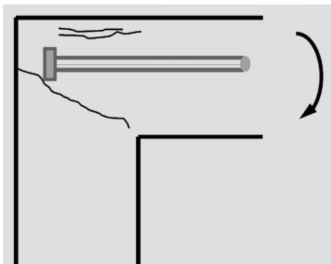
**Figure 7.** Knee joint with headed beam reinforcement.
