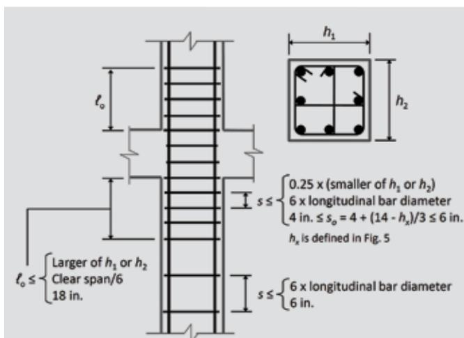
**Figure 4.** Confinement of rectangular column of special moment frame. Note:  $h_1$  = plan dimension of column in one of two orthogonal directions;  $h_2$  = plan dimension of column in other orthogonal direction;  $l_c$  = length, measured from joint face along axis of member, over which special transverse reinforcement must be provided;  $s$  = center-to-center spacing of items, such as longitudinal reinforcement, transverse reinforcement, tendons, or anchors. 1 in. = 25.4 mm.
