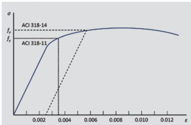
**Figure 16.** Definition of yield strength of high-strength reinforcement. Note:  $f_y$  = specified yield strength for nonprestressed reinforcement;  $\epsilon$  = strain in reinforcement;  $\sigma$  = stress in reinforcement.
